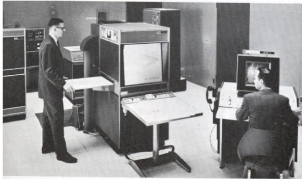
Figure 3.7 DAC-1 Hardware Configuration with Photo Scanner/Recorder at Center
